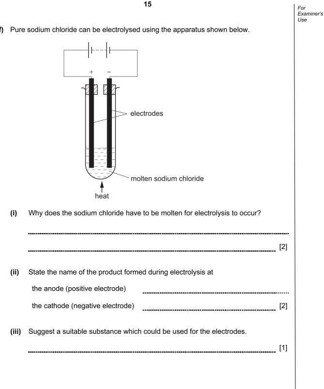
(f) Pure sodium chloride can be electrolysed using the apparatus shown below.
